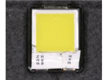
Figure 2. Example of a Damaged Silicone Resin
