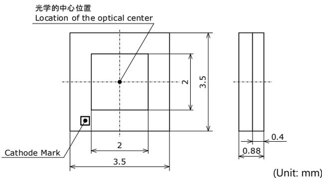
Figure 2. Outline Dimensions of the NVSW719AC LED
