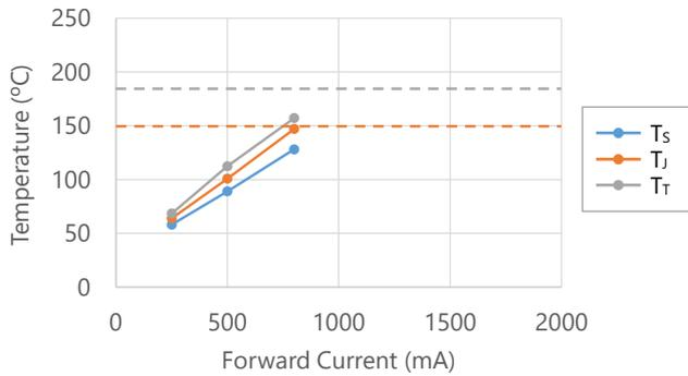
Figure 27. Measurement Results of Module 1 (Φ20mm)
