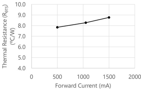
Figure 23. Measurement Results of the LEDs with Rank of sm27/R9050
