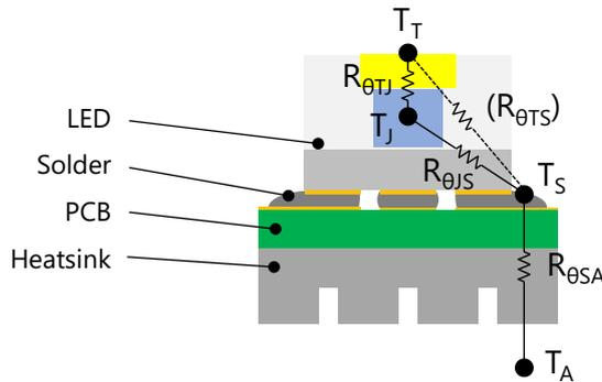
Figure 5. Thermal Resistance Model for the NVSW719AC LED
