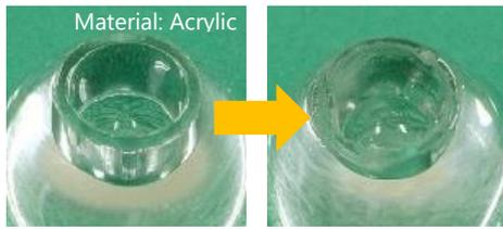
Figure 9. Example of Deformation of a Secondary Optical Lens due to Heat
