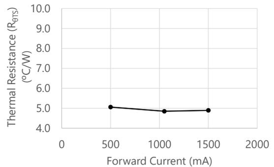
Figure 26. Measurement Results of the LEDs with Rank of Cr70/Rnn
