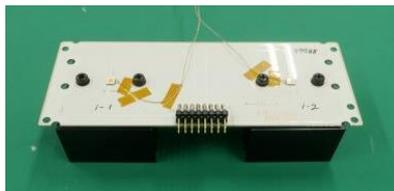
Figure 18. PCB and Heatsink Used for the Evaluation
