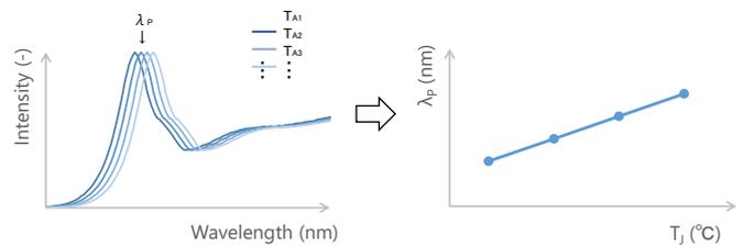
Figure 13. Relationship Between the Junction Temperature and the Peak Wavelength
