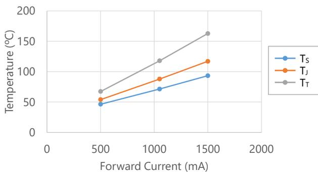
Figure 21. Measurement Results of the LEDs with Rank of sm50/R9050
