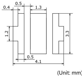
Figure 7. Recommended Soldering Pad Pattern
