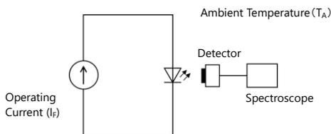
Figure 14. LED Chip's Peak Wavelength Measurement
