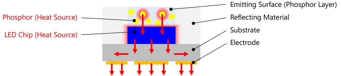
Figure 4. Reference Image of the Structure and Thermal Paths
