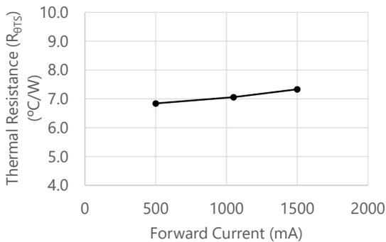
Figure 25. Measurement Results of the LEDs with Rank of sm50/R9050
