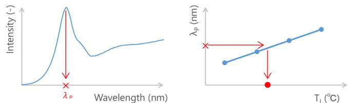
Figure 15. How to Obtain the LED Junction Temperature
