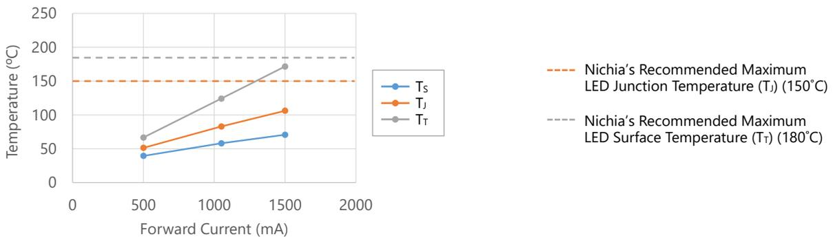
Figure 29. Measurement Results of Module 3 (Φ60mm)
