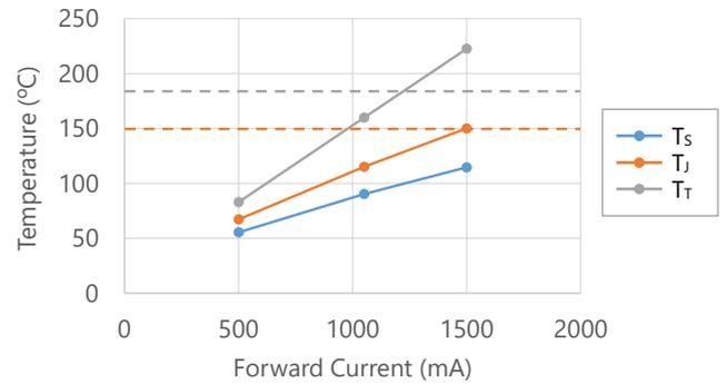
Figure 28. Measurement Results of Module 2 (Φ40mm)
