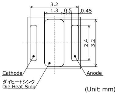
Figure 6. Electrodes on the LED Back Surface
