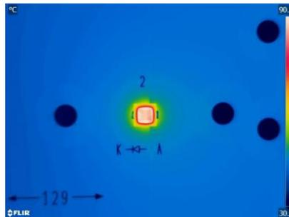
Figure 17. Example of Measurement Using a Thermal Imaging Camera
