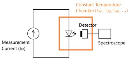
Figure 12. Measurement Circuit
