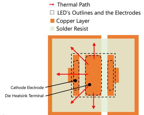
Figure 8. Example of Soldering Pad Pattern
