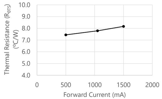
Figure 24. Measurement Results of the LEDs with Rank of sm40/R9050
