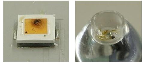
Figure 10. Examples of Burnt LED Emitting Surface and Secondary Optical Lens due to Flux Attached
