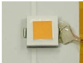
Figure 11. Example of How a Thermocouple is Attached with an Adhesive
