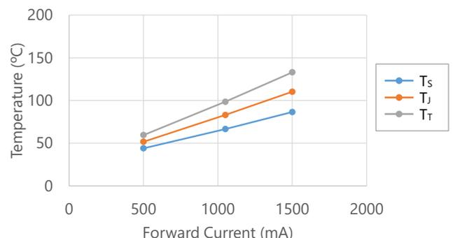
Figure 22. Measurement Results of the LEDs with Rank of Cr70/Rnn
