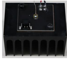
Picture 6. Fins facing down (This orientation obstructs the air flow)
