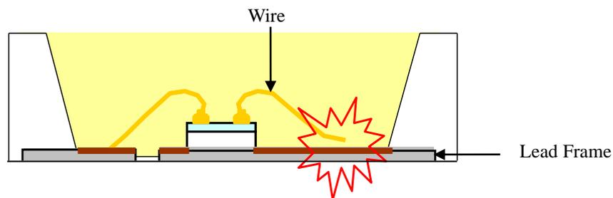
Figure 1-4. How Wire Breakage occurs due to Corrosion
