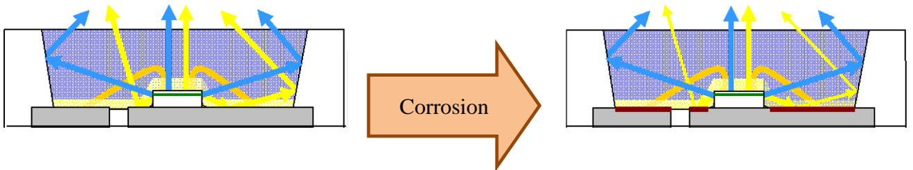
\*When the lead frame becomes discolored, the amount of reflected light at the lead frame surface decreases and it changes the spectrum distribution of the LED.
