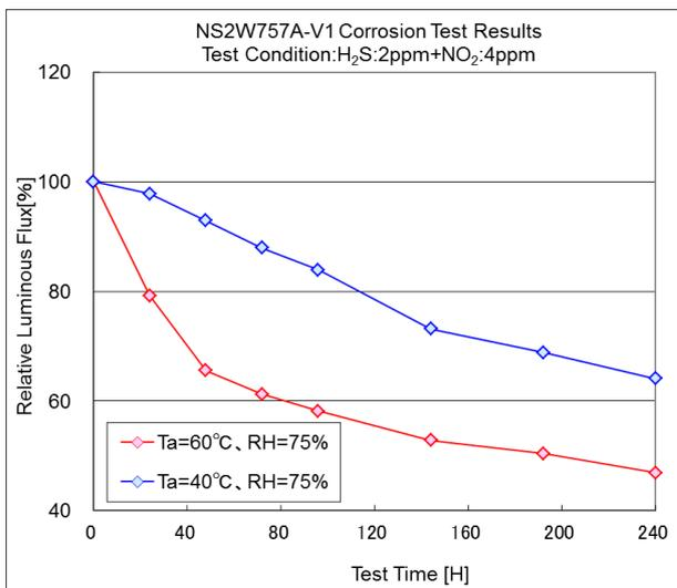
Figure 2-5. Mixed Gas Corrosion Test Results
