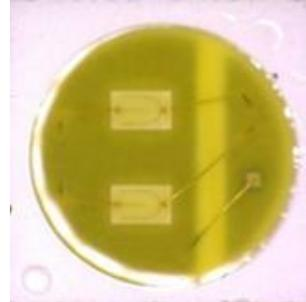
After being exposed to a corrosive environment containing sulfur
