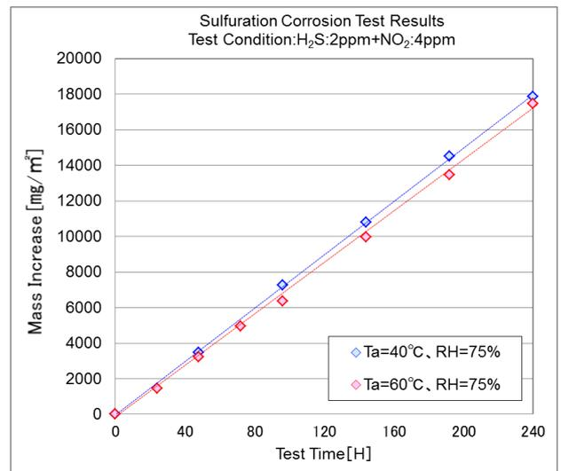
Figure 2-6. Mixed Gas Corrosion Test Results
