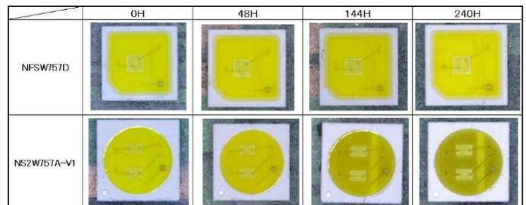
Figure 2-2. LED Accelerated Corrosion Test Results using the Improved Test Method
