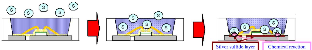
Figure 1-1. Schematic diagram of how sulfur causes a silver-plated lead frame to corrode (discolor)
