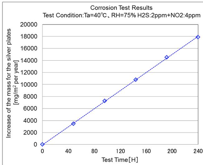
Figure 2-3. Increase in the Mass of the Silver Plates during the Corrosion Test
