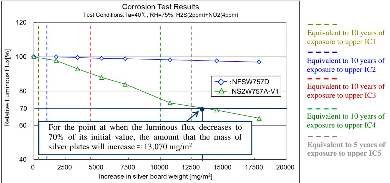
Figure 2-4. Estimated Lumen Maintenance Curves for NFSW757D and NS2W757A-V1
