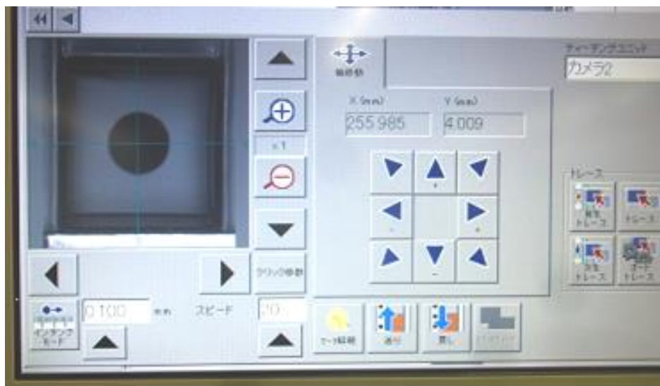
Figure 3. Yamaha YS mounter's pick-up nozzle positioning screen (Reference)
