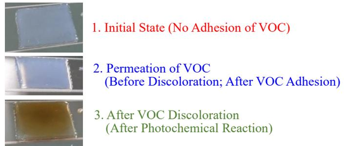
Figure 5. Transparency Change due to VOC Adhesion and Discoloration
