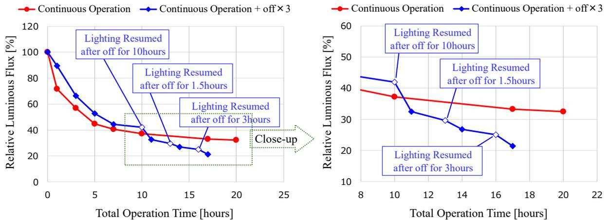
Figure 14. Comparison of Continuous Operation and On/Off Operation
