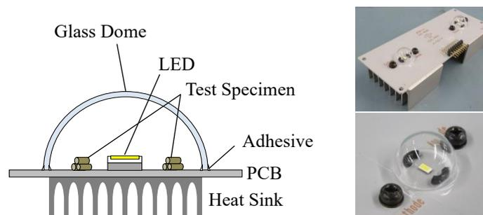
Figure 9. Example of Test Apparatus for VOC Discoloration Test
