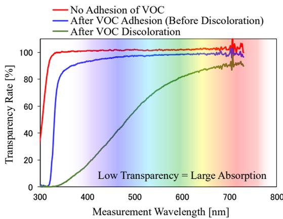
A silicone resin was applied to a glass plate and a VOC was adhered to the resin to compare changes in the condition of the resin.
