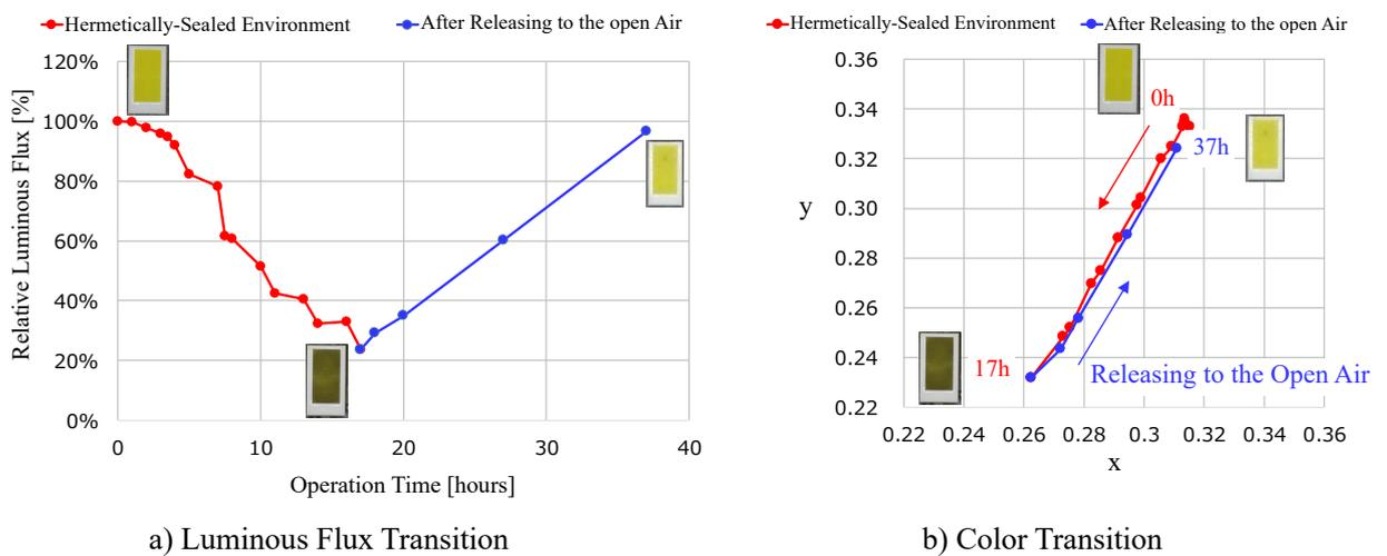
Figure 12. Discoloration of VOCs and Reduction in the Discoloration (Verification by Accelerated Test Under High VOC Concentration)
