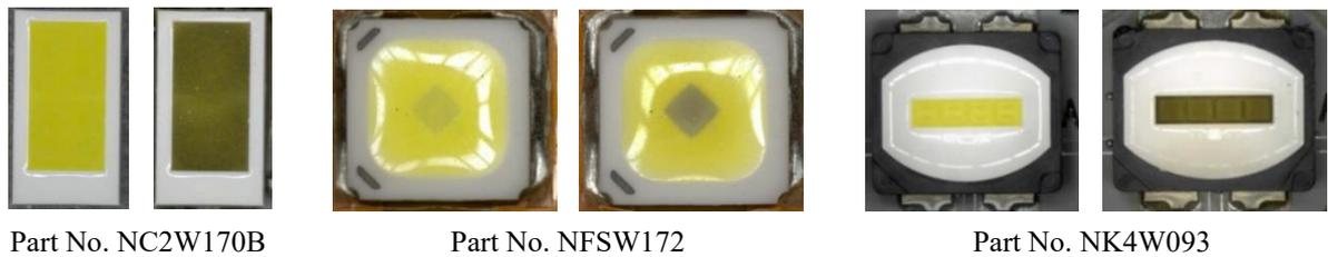
Figure 1. Adverse Effect of VOCs on LEDs (Left: Before Discoloration; Right: After Discoloration)
