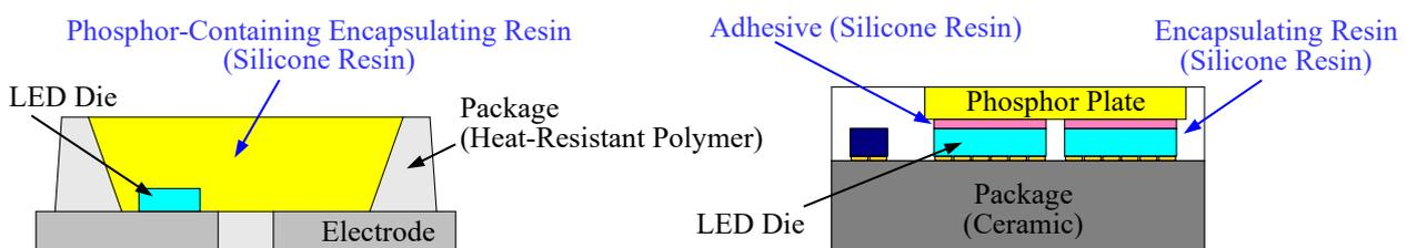
Figure 3. Examples of Silicone Resins Used in LED
