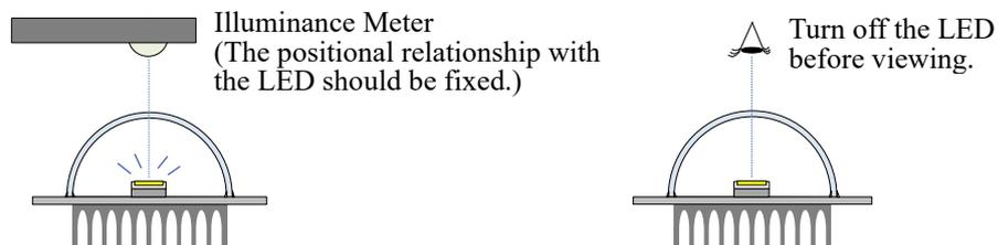
Figure 11. How to Check Luminous Intensity and Discoloration
