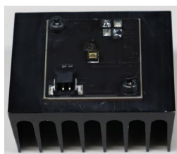
Picture 5. Fins facing down (This orientation obstructs the air flow)
