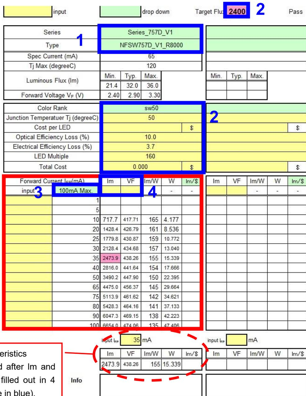
Characteristics obtained after I<sub>m</sub> and V<sub>F</sub> are filled out in 4 (enclose in blue).
