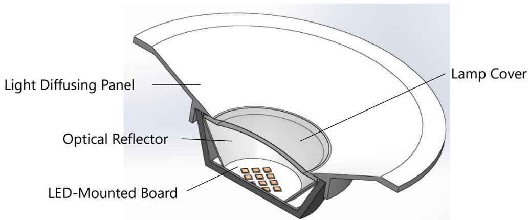
Figure 6. LED Tube Structure
