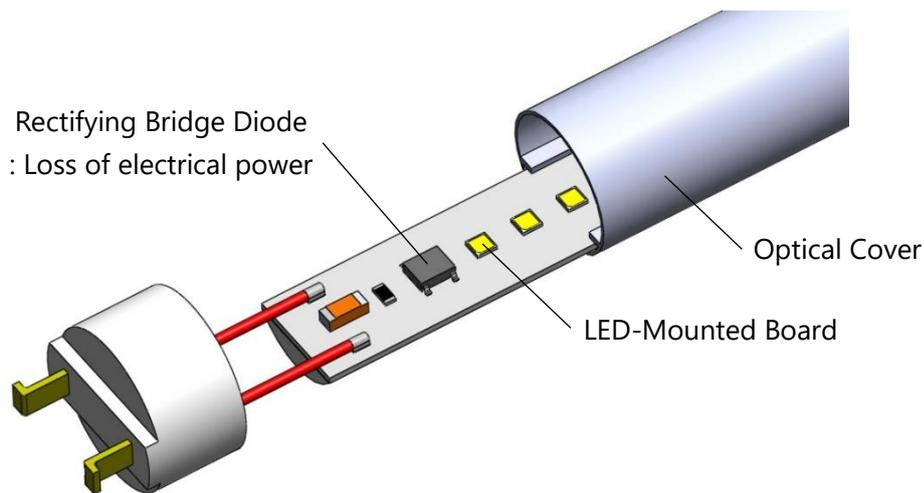
Figure 1. LED Tube Structure
