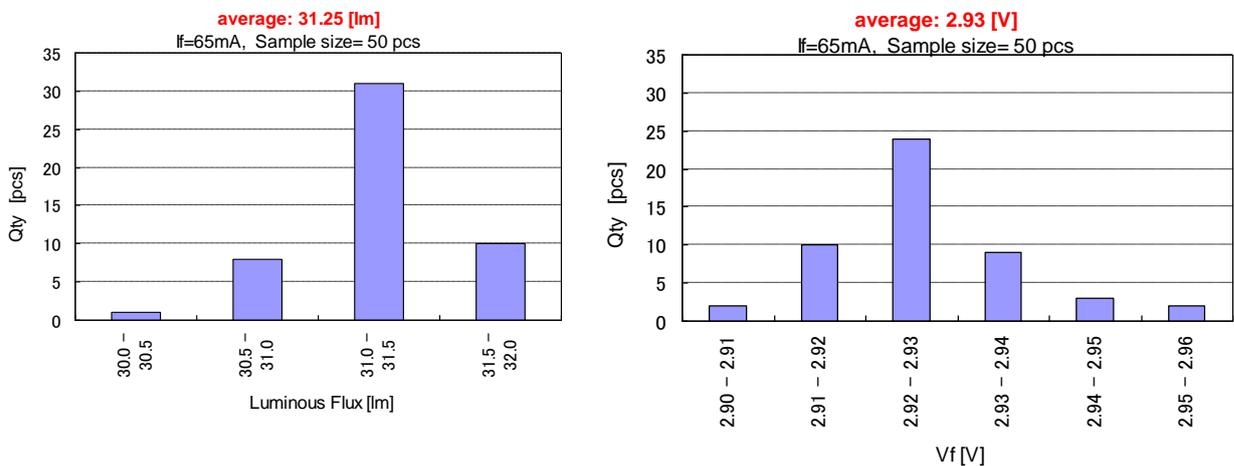
Figure 3. LED's Luminous Flux and VF (50 Sampled-out LEDs)
