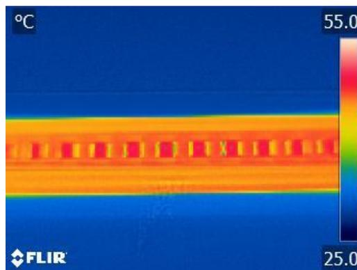
Figure 4. Thermal Distribution in the LED Tube
