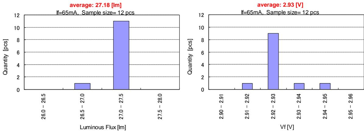
Figure 8. LED's Luminous Flux and V<sub>F</sub> (12 LEDs)
