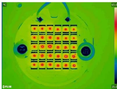
Figure 4. Example of an Even Temperature Distribution
