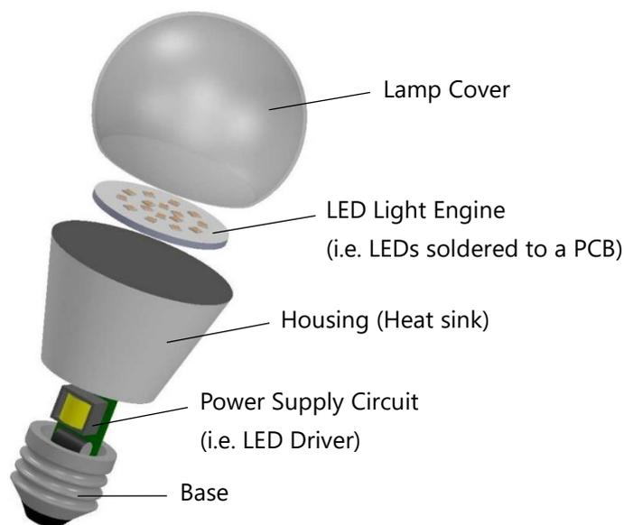
Figure 1. Structure of a Typical LED retrofit lamp
