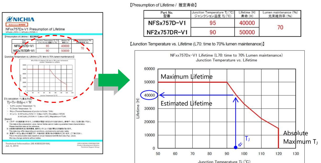
Figure 3. Example of the Technical Data (NFSx757D-V1/NF2x757DR-V1 Presumption of Lifetime)
