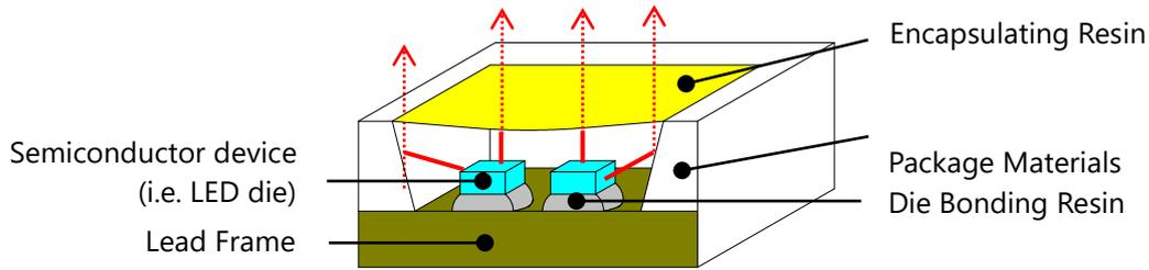
Figure 2. Internal Structure of a NICHIA 757 series LED
