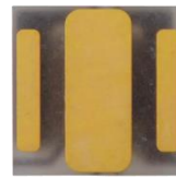
NVSW219F-V1 Bottom Surface (Three Electrodes)
