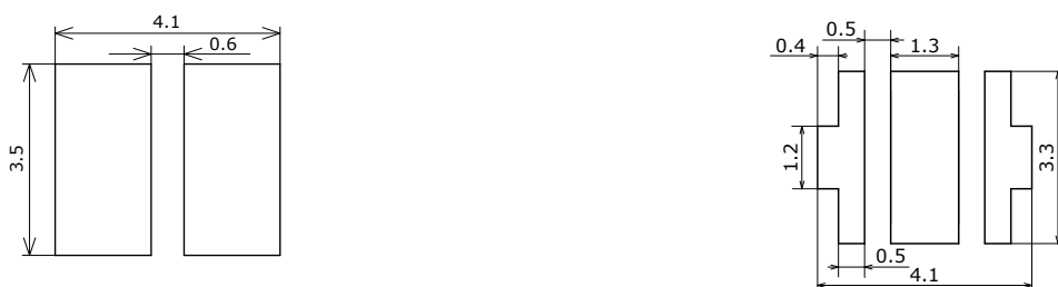
NICHIA 119 series (two-electrode configuration) NICHIA 219 series (three-electrode configuration) Figure 5. LED recommended soldering pad pattern
