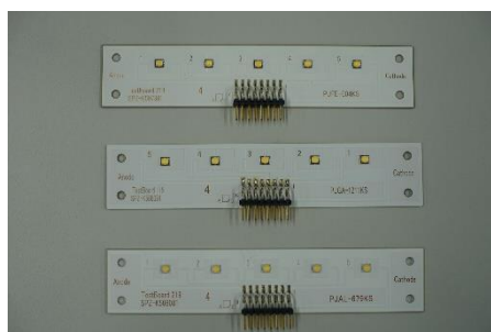
Figure 6. Example of how the LEDs were mounted on the PCB
