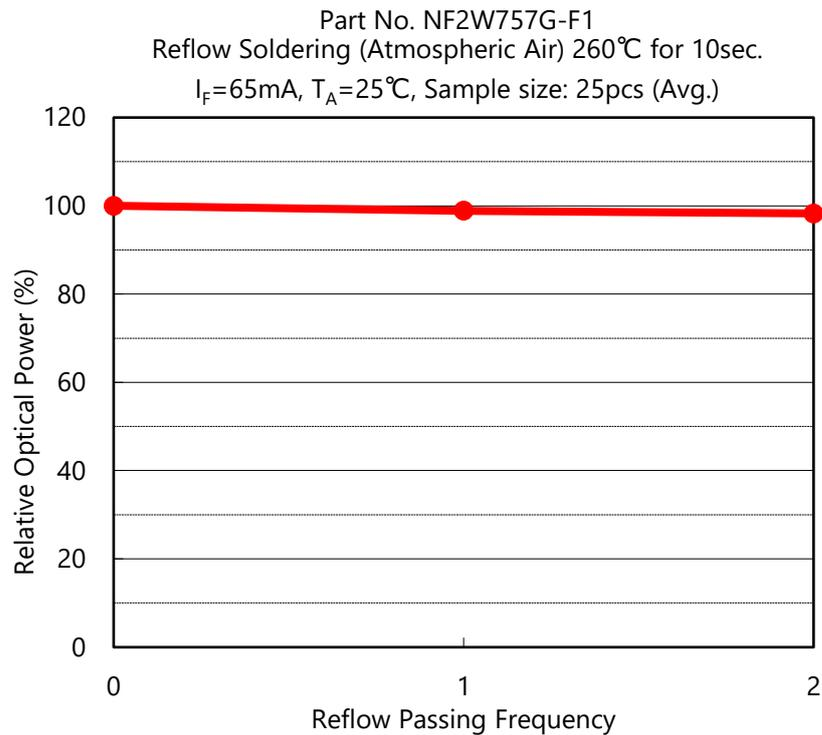
Figure 22. Luminous flux reduction rate confirmation data in air reflow (example: part number NF2W757G-F1)
