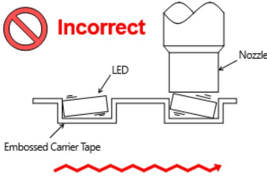
Figure 9. Tape feeder with large vibration
