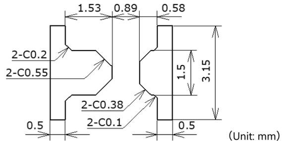
Figure 2. Example metal solder stencil aperture as a countermeasure against part floating
