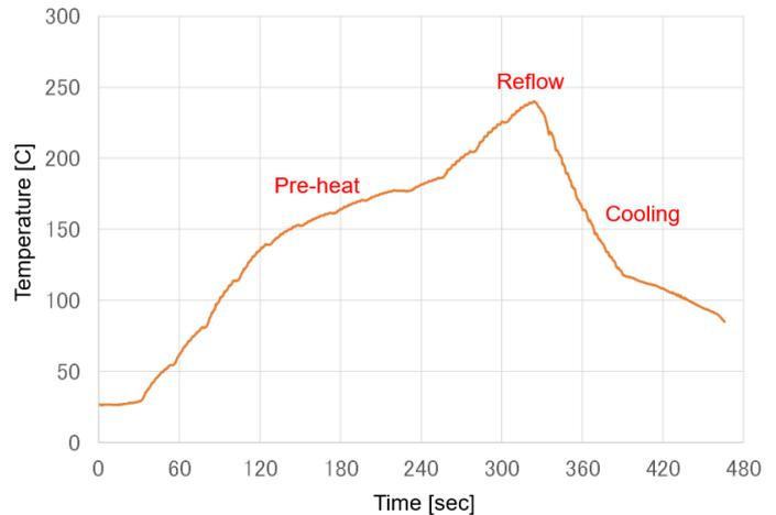
Figure 20. Example of a Reflow Profile
