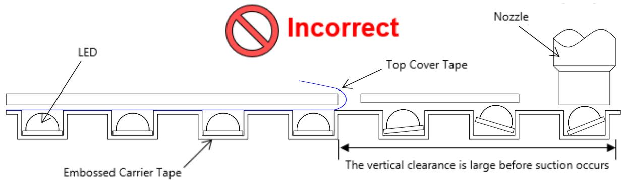
Figure 15. Removing the top cover tape in the normal position
