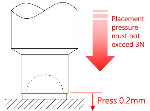
Figure 18. Nozzle Placement Depth
