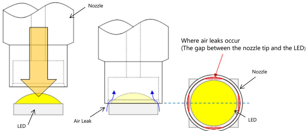
Figure 8. Air leak at the time of LED suction (example: part number NV9W149AM)
