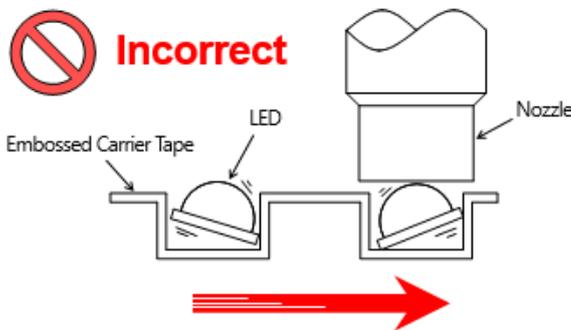
Figure 11. Tape feeder feed rate (fast)
