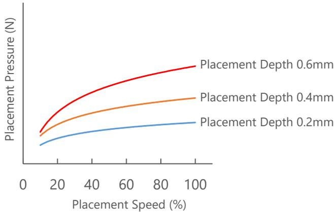
Figure 17. Placement pressure due to placement depth
