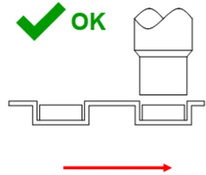
Figure 10. Tape feeder with small vibration
