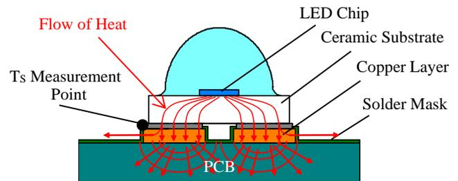
Figure 5. Thermal Path of the NVSx119C LEDs
