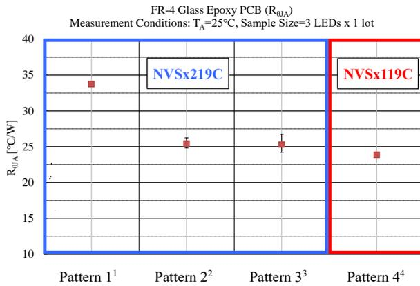
**Figure 6. Evaluation Results for the Thermal Resistance ( $R_{\theta JA}$ )**
