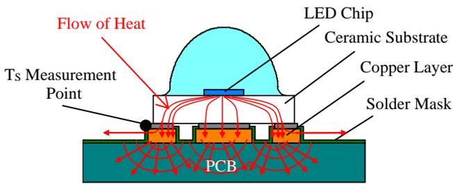
Figure 4. Thermal Path of the NVSx219C LEDs
