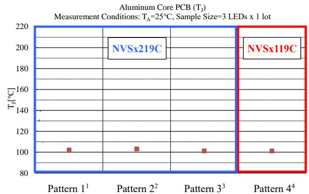
Figure 9. Evaluation Results for the Junction Temperature ( $T_j$ )
