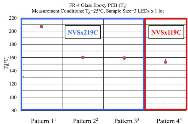
**Figure 7. Evaluation Results for the Junction Temperature ( $T_J$ )**
