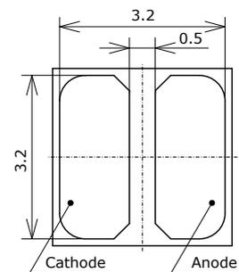
Figure 1. Appearance of the NVSxx19C series LEDs
