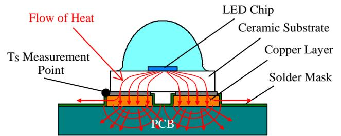
Figure 5. Thermal Path of the NVSx119C LEDs
