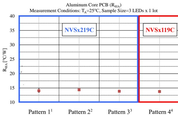
Figure 8. Evaluation Results for the Thermal Resistance ( $R_{\theta JA}$ )
