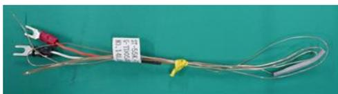
Figure 12. Example of a Thermocouples used by Nichia
