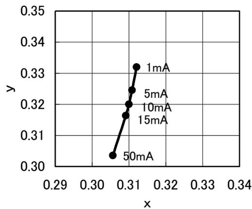
Figure 2. Forward current vs. Chromaticity NECW425B
