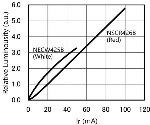
Figure 1. Forward Current vs. Relative Luminosity of NECW425B and NSCR426B
