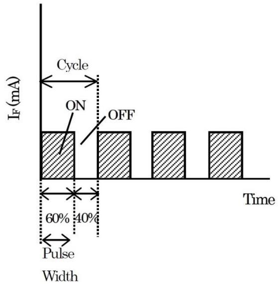
Figure 4. Pulse-width modulation (PWM)
