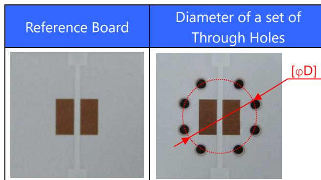
Please refer to Figure 4 for the evaluation results of the heat dissipation depending on the diameter of a set of Through Holes.
