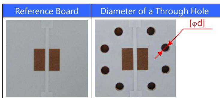
The heat dissipation in each condition is evaluated by the ratio of  $T_J$ , regarding the  $T_J$  of the reference board without any Through Hole as 1. Please refer to Figure 2 for the evaluation results of the heat dissipation depending on the diameter of a Through Hole.
