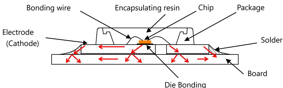
Figure 1. Cross Section of LED and Thermal Path
