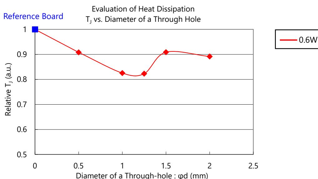
Figure 2. Evaluation Result of Heat Dissipation Depending on Diameter of a Through Hole
