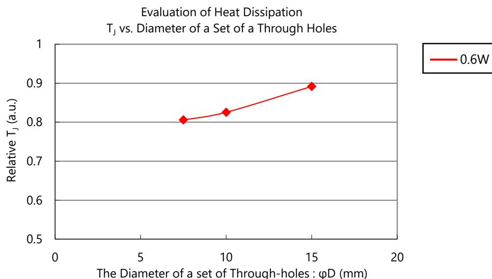
Figure 4. Evaluation Result of Heat Dissipation Depending on the Diameter of a Set of Through Holes
