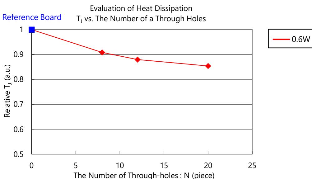
Figure 3. Evaluation Result of Heat Dissipation Depending on the Number
