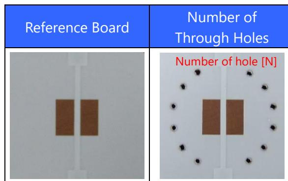
Please refer to Figure 3 for the evaluation results of the heat dissipation depending on the number of Through Holes.
