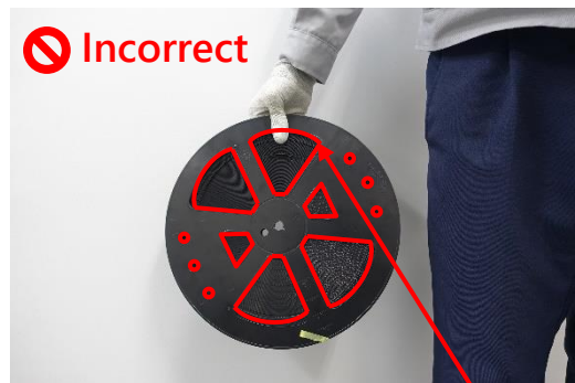
Do not hold the reel where the tape is exposed.
