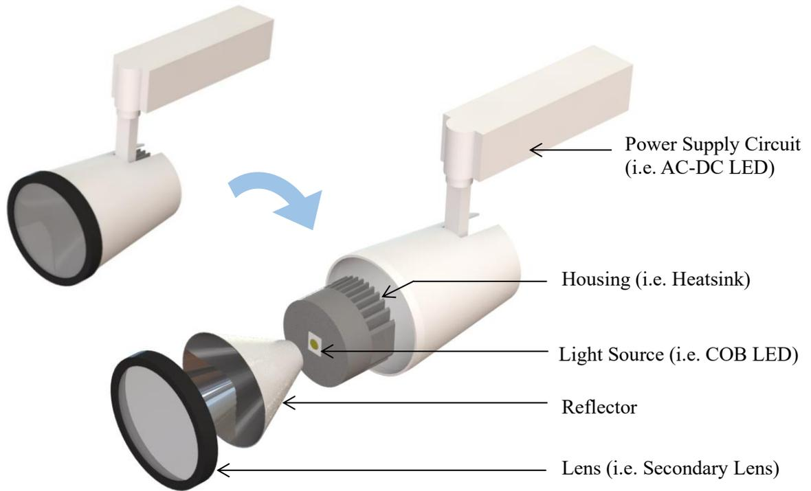
Figure 1. Structure of a typical COB-based spotlight
