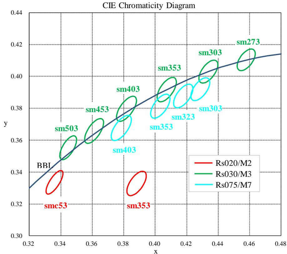
Figure 6. Color Ranks for the Special Color Rendering COB LEDs
