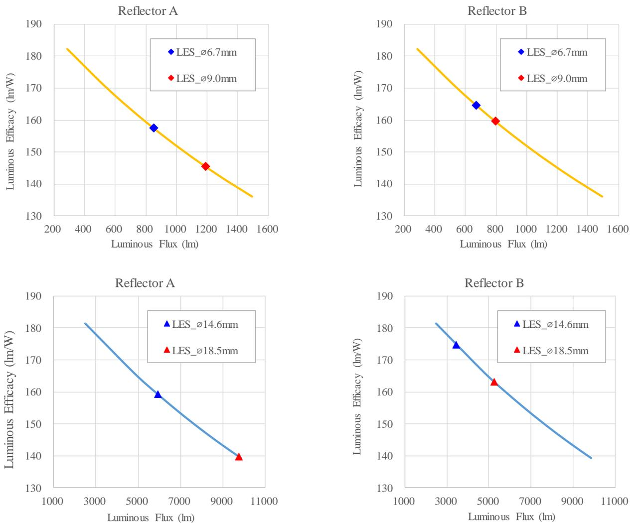
Figure 4. Advantages of COB LEDs with a small LES in increasing the luminous efficacy (lm/W) of the modules when operated so that the center luminous intensity values are the same ( $T_J=85^{\circ}\text{C}$ )
