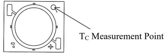
Figure 5. Position of the  $T_C$  measurement point
