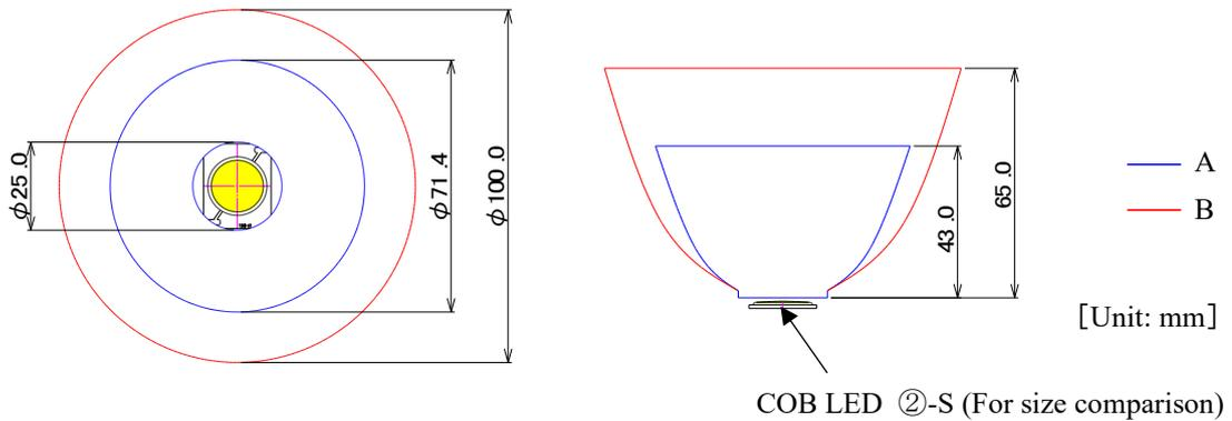
Figure 3. Outline Dimensions of the Reflectors
