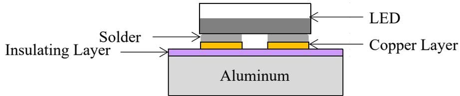
Figure 3. Step 1: Soldering an LED to an aluminum-core PCB
