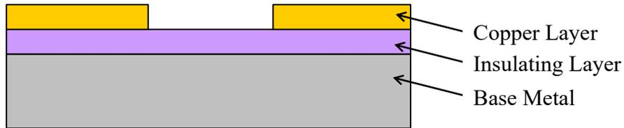
Figure 6. Structure of the metal-core test PCB
