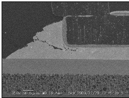
Figure 1. Example of a Solder Crack
