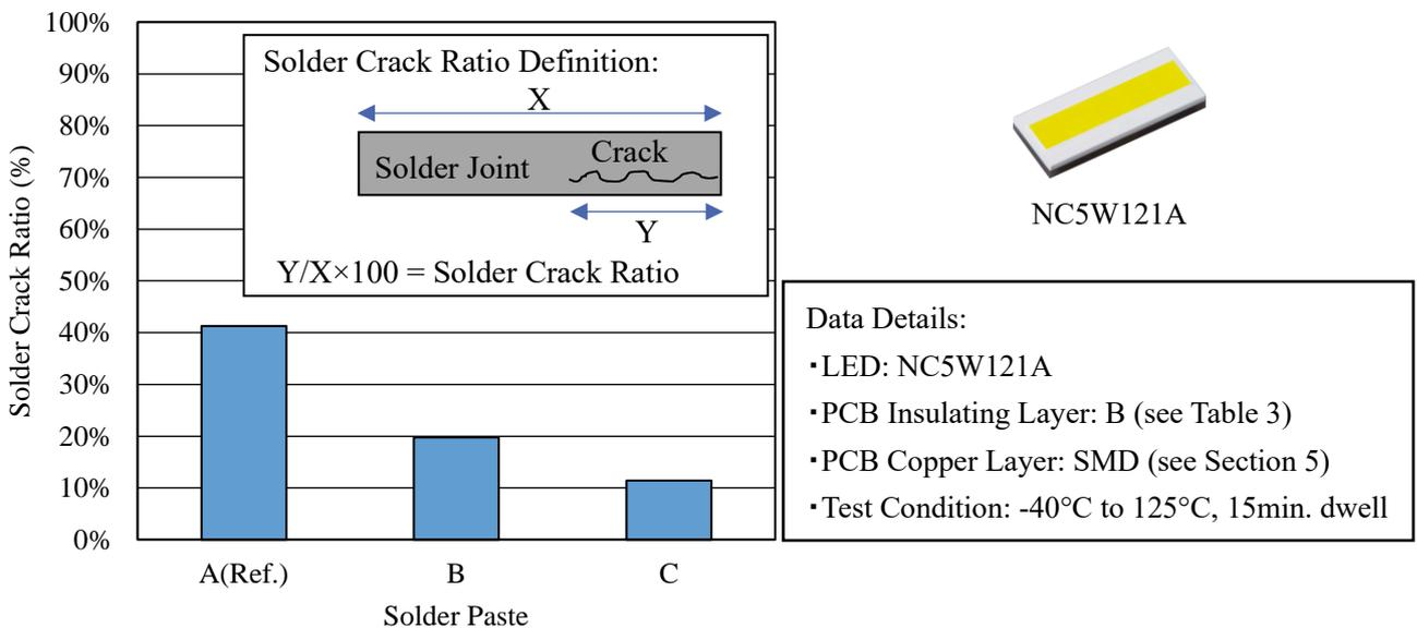
Figure 9. Solder crack resistance via thermal shock test
