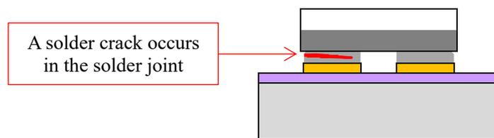
Figure 5. Step 3: Solder cracks occur
