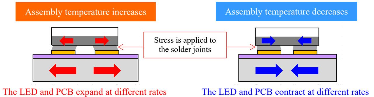
Figure 4. Step 2: The LED and PCB expand and contract at different rates
