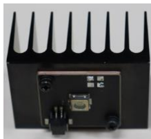
Picture 8. Fins facing vertical (Nichia uses this orientation)
