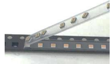
Figure 18. LED Sticking due to Static Charge
