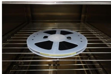
Figure 5. Example for Baking the LEDs
