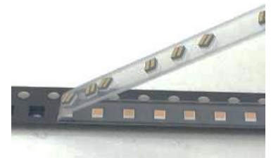
Figure 16. LED Sticking due to Static Charge
