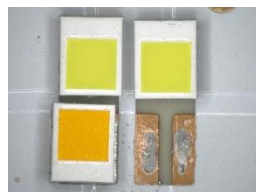
b) Solder Printing Failure Resulting in Open Circuit/LED Removal from the PCB
