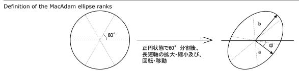
A perfect circle is divided into 60 degree-sections and then transformed into the MacAdam ellipse that is presented on the chromaticity diagram in this specification.
